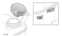
Ensure the coolant level remains between the **MIN** and **MAX** indicator marks on the side of the expansion tank.
