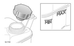
Ensure the coolant level remains between the **MIN** and **MAX** indicator marks on the side of the expansion tank.
