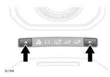
Terrain Response selection is via center console switches. Use the switches to move through up the five program selections. The currently selected program icon will be displayed in the message center.
