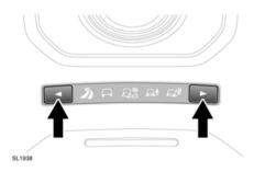
Terrain Response selection is via center console switches. Use the switches to move through up the five program selections. The currently selected program icon will be displayed in the message center.
