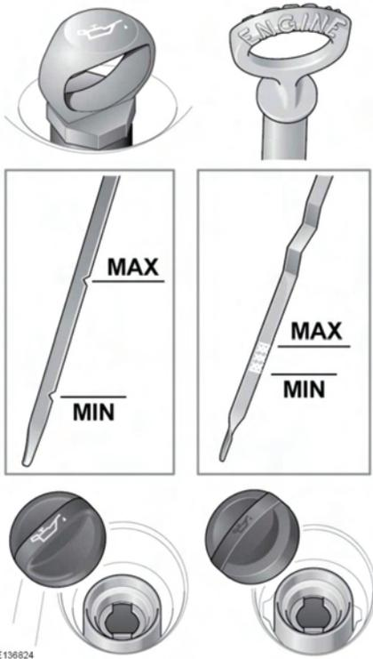
1. Withdraw the dipstick and wipe the blade clean with a lint free cloth.
