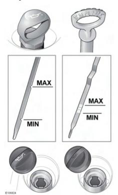
1. Withdraw the dipstick and wipe the blade clean with a lint free cloth.
