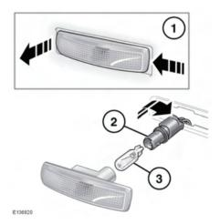
Follow the steps illustrated. Insert a new bulb and refit the components.
