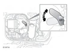
Note: The headlamps must be removed in order to change the beam pattern. See 147, HEADLAMP REMOVAL146, CHANGING A BULB.
