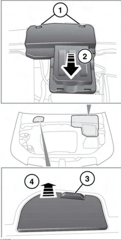
1. Press the tabs to release the cover from the casing.
