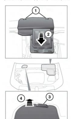
1. Press the tabs to release the cover from the casing.
