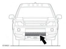
Ensure that the areas around air intakes and the front grille are clean and clear of debris. Pay particular attention to the lower grille and radiator. Failure to do so may cause the engine to overheat, leading to severe engine damage.
