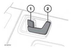
From inside the vehicle, all the doors can be locked by pressing either the driver or passenger lock lever (1).
