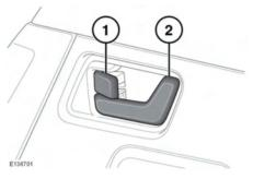
From inside the vehicle, all the doors can be locked by pressing either the driver or passenger lock lever (1).
