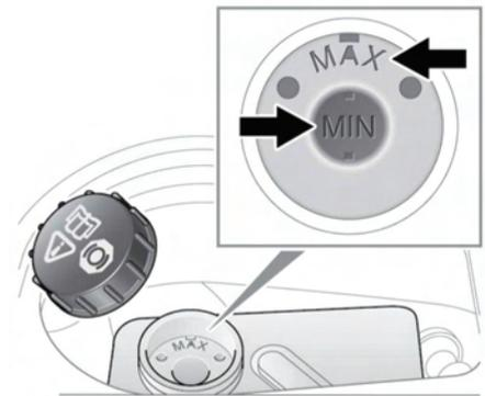
1. Clean the filler cap before removing to prevent dirt from entering the reservoir.
