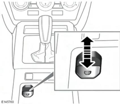
With the ignition turned on, press the brake pedal and press down on the EPB switch. This will release the electronic parking brake.
