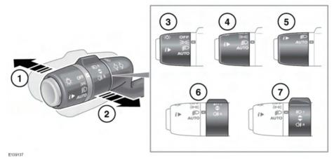
With the headlamps on, push the control away from the steering wheel to select high beam. The warning lamp will illuminate. See 49, HIGH BEAM (BLUE).
