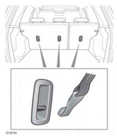
**Note:** A tether anchorage is provided for the centre seat position. Do not use this anchor position with an ISOFIX child seat.
