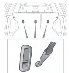
**Note:** A tether anchorage is provided for the centre seat position. Do not use this anchor position with an ISOFIX child seat.
