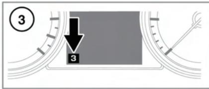
To use CommandShift™, first select sport mode, then move the selector lever forward to move up a gear, and back to move down gear.
