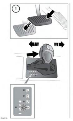
**1.** To select Drive (**D**) when the vehicle is stationary, apply the foot brake and press the gear selector release button.
