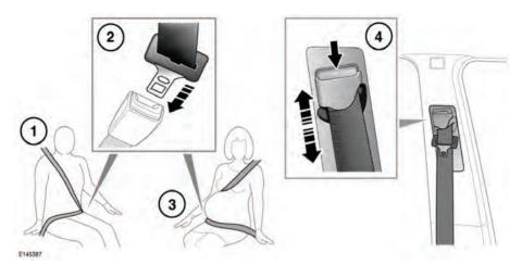
PUTTING ON A SEAT BELT: Draw the belt out smoothly and ensure that the belt height, the seat and your position on the seat, are correct.
