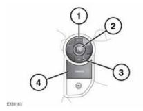
SET+: Press to set the speed or to increase the set speed. The cruise control warning lamp will illuminate to confirm cruise control is operational (see 61, CRUISE CONTROL (GREEN)).
