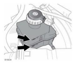
The driver's side cover must be removed to check the brake fluid level. See 199, UNDER BONNET COVERS - REMOVAL.
