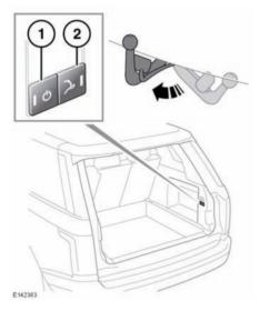
The electrically deployable tow bar is hidden in its stowed position behind the bumper. It can be deployed using the buttons located on the right side of the loadspace.
