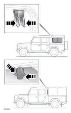
Squeeze either type of lock and slide the window to the desired position. Release the lock and ensure that the catch is located securely into a locking socket.
