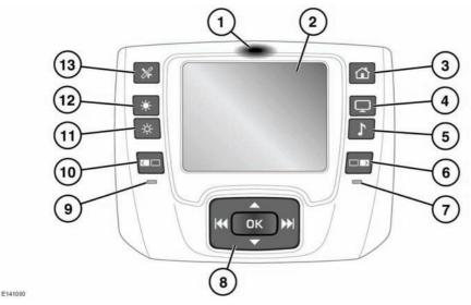
**Note:** The rear media remote control communicates via infra-red and must be pointed towards the receiver in the rear screen.
