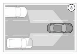
The Blind Spot Monitor (BSM) system monitors a zone that covers the area adjacent to the vehicle, that is not easily visible by the driver and is designed to identify any object overtaking the vehicle (3). The system uses a radar on each side of the vehicle to identify any overtaking vehicle/object within the blind spot area of the vehicle, while disregarding other objects which may be stationary or travelling in the opposite direction.
