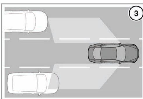
If an object is identified by the system as being an overtaking vehicle/object, an amber warning indicator icon (1) illuminates in the relevant exterior mirror, to alert the driver that there is a potential hazard in the vehicle's blind spot and therefore, that a lane change might be dangerous.
