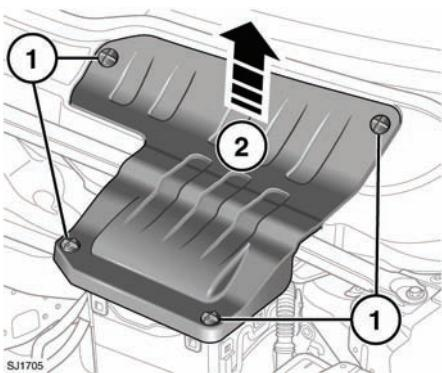
1. Turn the four fasteners 90 degrees counter-clockwise to release.
