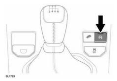
To switch the system off (preventing automatic stop/start) press the **ECO** switch. The amber LED indicator will extinguish to confirm that the system is off.
