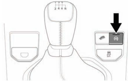
To switch the system off (preventing automatic stop/start) press the **ECO** switch. The amber LED indicator will extinguish to confirm that the system is off.
