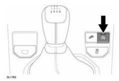
To switch the system off (preventing automatic stop/start) press the **ECO** switch. The amber LED indicator will extinguish to confirm that the system is off.
