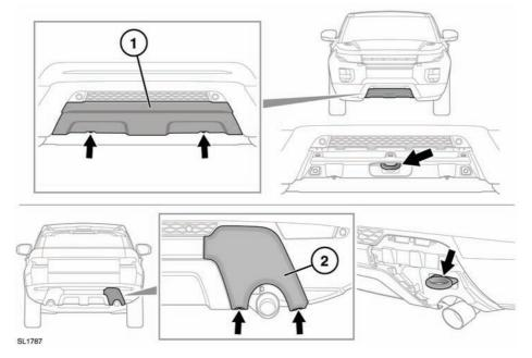
The towing eyes are located behind panels in the bumpers. Panel design will vary depending on the vehicle specification. To use the towing eyes:
