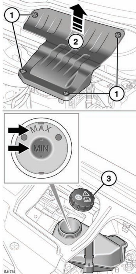
1. Remove the battery cover. Turn the four fasteners 90 degrees counter-clockwise to release.
