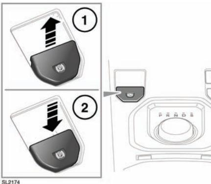
1. To apply the parking brake while the ignition is on or off, with the vehicle stationary pull up the lever and release it.
