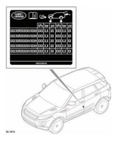
The recommended tyre pressures are listed on the tyre pressure label. See **245**, **LABEL LOCATIONS**
