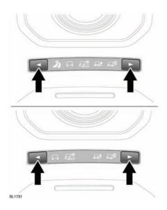
Terrain Response selection is via one of two centre console switches. Depending on vehicle specification, the control switches may include a Dynamic program setting. Use the switches to move through up to five program selections. The currently selected program icon will be displayed in the message centre.
