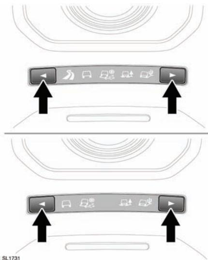
Terrain Response selection is via one of two centre console switches. Depending on vehicle specification, the control switches may include a Dynamic program setting. Use the switches to move through up to five program selections. The currently selected program icon will be displayed in the message centre.
