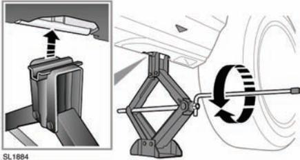
1. Locate the jack under the relevant jacking point.
