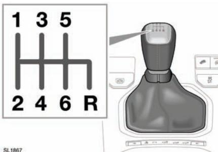
**!** Selection of reverse gear is prevented when the vehicle is travelling in excess of 24km/h (15mph). Never attempt to engage reverse gear while the vehicle is in forward motion. This may result in serious transmission damage and costly repairs.
