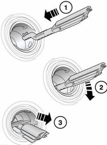
Reset the misfuel protection device as follows:
