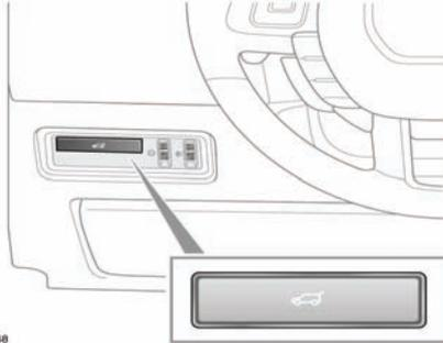
Both types of tailgate can be released using:
