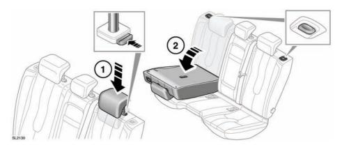
The split fold rear seat of 5 door models can be folded completely, or partially at 60/40 split, to accommodate loads and still retain seating for passengers.
