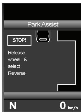
6. An instruction to select reverse gear will follow. Park assist will then take control of the vehicle's steering system so you must release the steering wheel. Apply the accelerator carefully to move the vehicle slowly into the parking space. Use the foot brake when instructed to do so.
