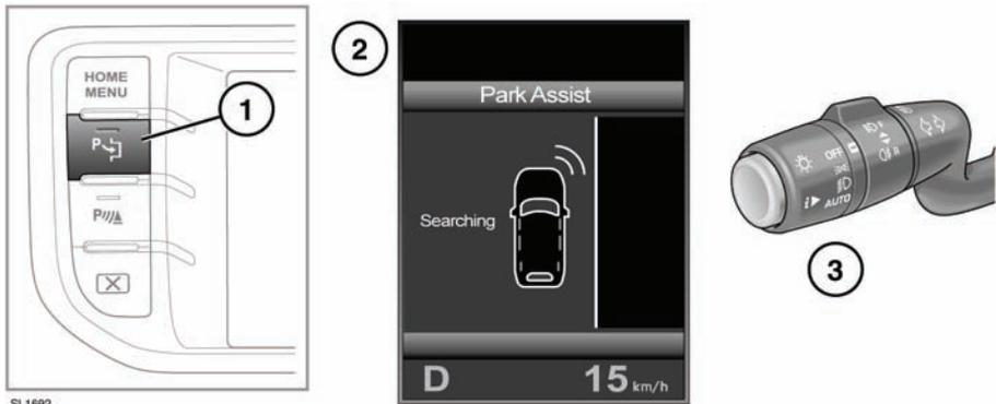
1. To activate, press the Park assist button while driving forwards at less than 30 km/h (19 mph). The indicator lamp in the button illuminates.
