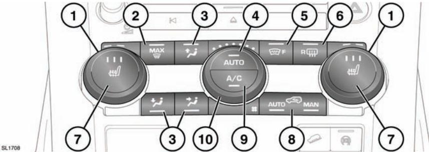
1. Temperature controls. For individual driver/passenger settings.
