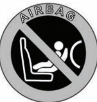
This symbol, affixed to the end of the fascia on the passenger side, warns against the use of a rear-facing child seat in the front passenger seat, when a front passenger airbag is fitted and operational.
