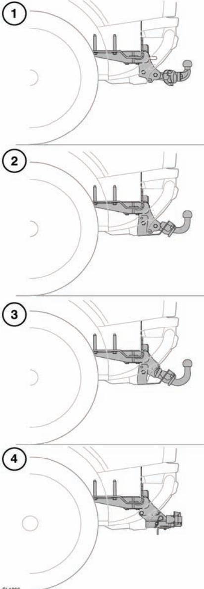
1. Bolt on tow ball onto flange.
