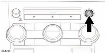
Press to turn the hazard warning lamps on. Press again to turn off. When the hazard warning lamps are operating, the direction indicator warning lamps will flash in time with the hazard warning lamps.
