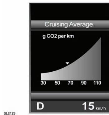
When enabled, a CO<sup>2</sup> emission indicator is displayed in the message centre. The higher the numeric reading, the more CO<sup>2</sup> is being emitted and the more fuel is being used. See **59, VEHICLE INFORMATION AND SETTINGS MENU**.
