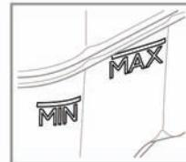
Ensure the coolant level remains between the **MIN** and **MAX** indicator marks on the side of the expansion tank.
