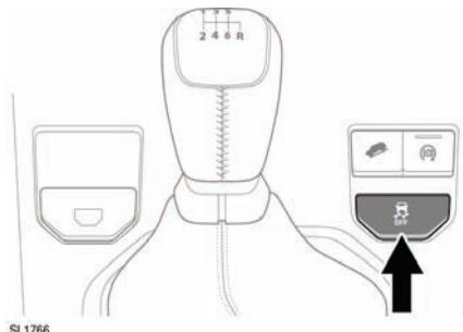
To disable DSC, press and briefly hold the DSC OFF switch. The DSC OFF warning lamp will illuminate continuously. The amber DSC OFF warning lamp in the instrument panel will also illuminate. See **63, DYNAMIC STABILITY CONTROL (DSC) OFF (AMBER)**. Deactivating DSC also reduces the level of electronic traction control intervention and may lead to an increase in wheel spin.
