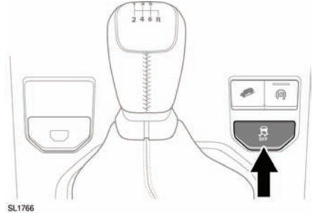
To disable DSC, press and briefly hold the DSC OFF switch. The DSC OFF warning lamp will illuminate continuously. The amber DSC OFF warning lamp in the instrument panel will also illuminate. See **63, DYNAMIC STABILITY CONTROL (DSC) OFF (AMBER)**. Deactivating DSC also reduces the level of electronic traction control intervention and may lead to an increase in wheel spin.
