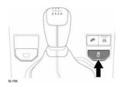
To disable DSC, press and briefly hold the DSC OFF switch. The DSC OFF warning lamp will illuminate continuously. The amber DSC OFF warning lamp in the instrument panel will also illuminate. See 63, DYNAMIC STABILITY CONTROL (DSC) OFF (AMBER). Deactivating DSC also reduces the level of electronic traction control intervention and may lead to an increase in wheel spin.
