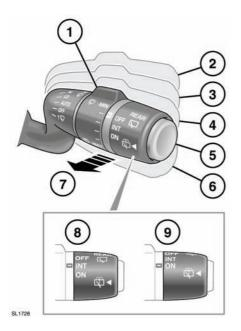
Rotate the collar to adjust the intermittent period. The intermittent delay period will vary and is controlled by either vehicle speed or a rain sensor. The control must be in position (4) to be operational.
