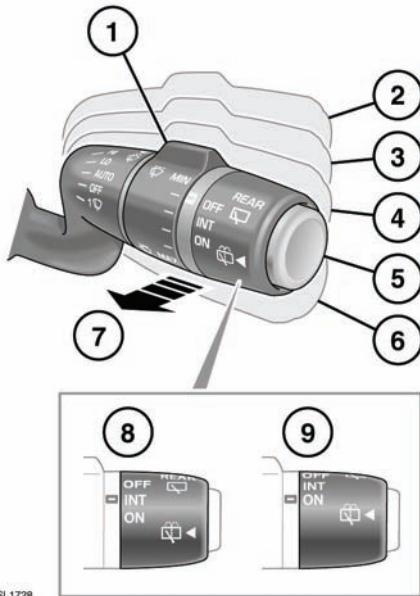
1. Rotate the collar to adjust the intermittent period. The intermittent delay period will vary and is controlled by either vehicle speed or a rain sensor. The control must be in position (4) to be operational.
