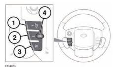
1. SET+: Press to set the speed or to increase the set speed. The cruise control warning lamp will illuminate to confirm cruise control is operational (see 55, CRUISE CONTROL (GREEN)).
