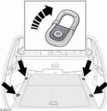
To assist in safely securing large items of luggage, four fixing points are located in the rear loadspace floor.
