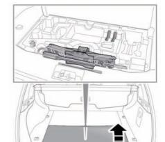
The tool kit is located under a panel set in the loadspace floor.
