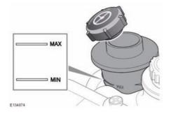
The level of fluid can be seen through the translucent body of the reservoir.
