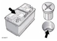
Unscrew the six cell plugs and store carefully. Check that the surface of the liquid (electrolyte) is level with the plastic level indicator. If necessary, top up with distilled water, but never overfill. Refit the six cell plugs.
